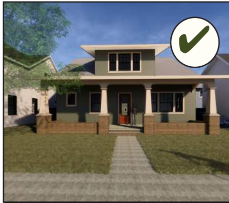
The masonry and smooth finished HardiePlank siding on this Craftsman-influenced house is appropriate for Haggard Park.
