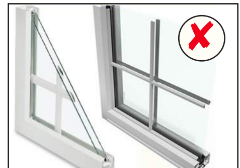
Illustration of vinyl window, showing muntins inappropriately applied to the glass.
