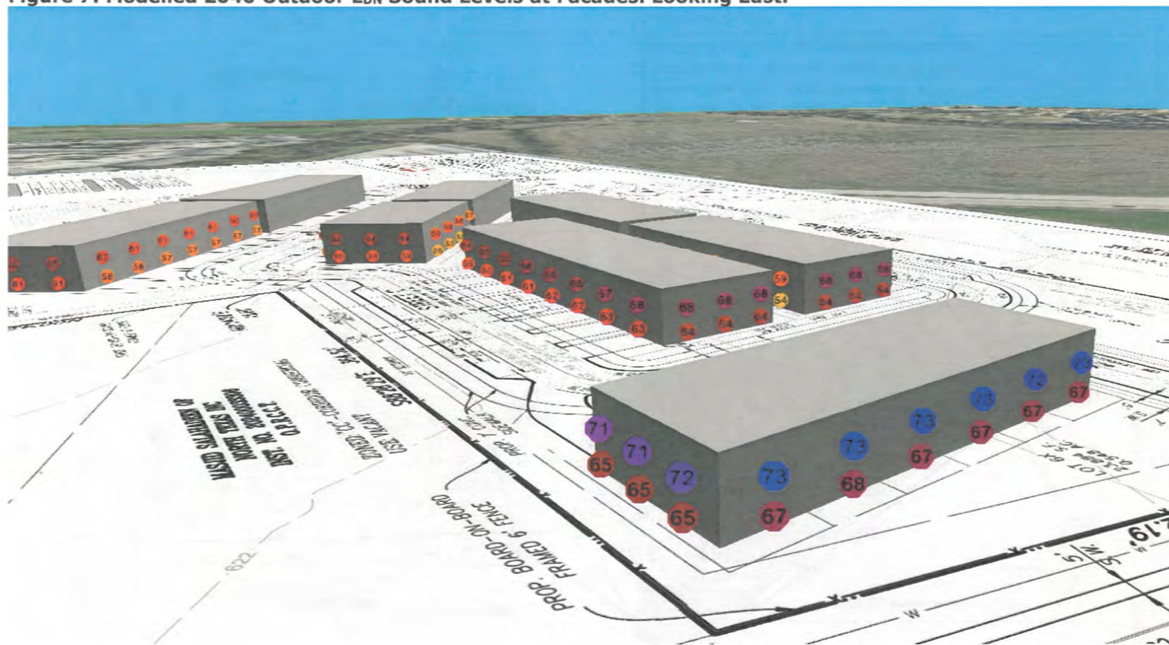
Figure 7: Modelled 2040 Outdoor L_{DN} Sound Levels at Facades. Looking East.
