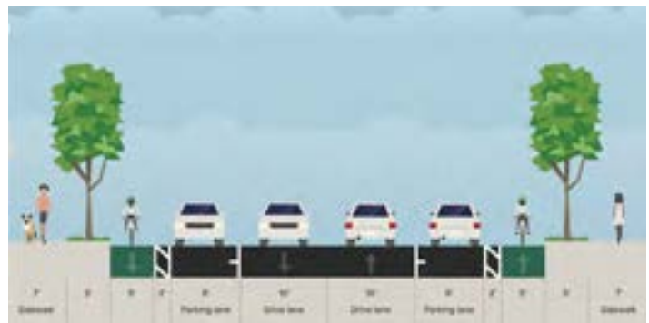
F Avenue – Southwestern Avenue to Plano Parkway On-Street Parking Lanes + Buffered Bike Lanes (74' ROW) (Long-Term Rebuild Solution)
