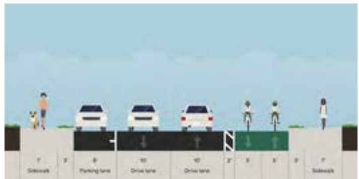
F Avenue – Southwestern Avenue to Plano Parkway On-Street Parking Lane + Buffered Cycle Track (60' ROW) (Short-Term Retrofit Solution)
