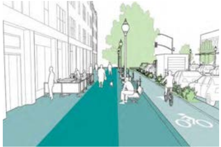
Pedestrian-oriented street elements: wide sidewalk, seating, lighting
